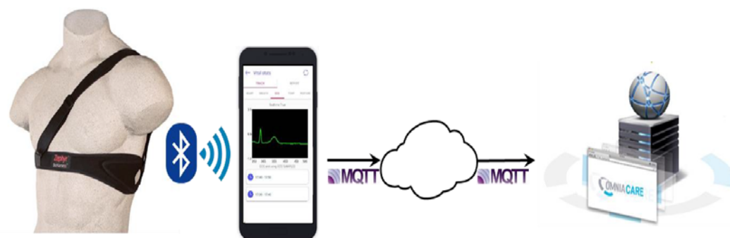
Fig.1. Data acquisition and transmission
